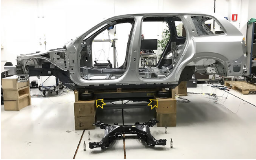
Fig. 5.18 Body in White chassis of a Volvo XC90 resting on rubber cushions (at yellow arrows) ready for vibration testing. Loose rear subframe resting on lab floor in front
