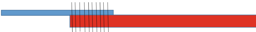
Fig. 4.1 Sample substructuring problem where two beams are joined by 10 bolts, represented by vertical lines
