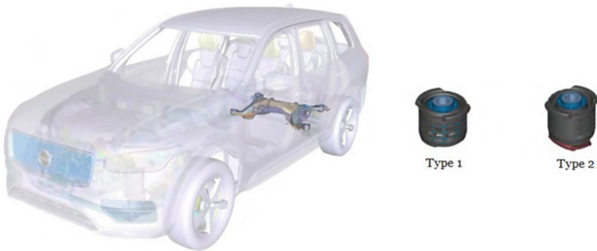
Fig. 5.9 Rear subframe location in the car and two bushing types of particular interest
